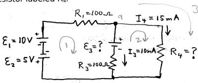
$KCL @ \Rightarrow I_1 - I_4 - I_3 = 0 \Rightarrow I_1 = I_3 + I_4 = 10 \text{ mA} + 15 \text{ mA} = 25 \text{ mA}$  $KVLD \Rightarrow 5V - R_1 I_1 - \epsilon_3 - I_3 R_3 = 0 \Rightarrow \epsilon_3 = 5V - 3.5V$
