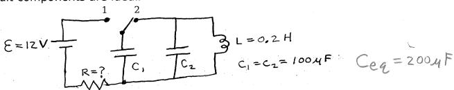
a) (2 pts) The switch is switched to position 1. The capacitor, C1, takes
