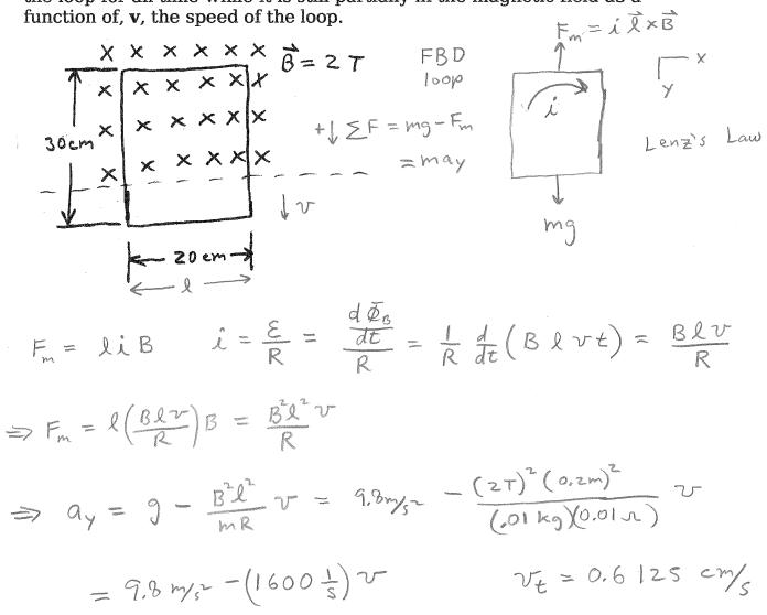
Direction (circle one) = counterclockwise clockwise  $a(0) = 9.8 \text{ m/s}^2$   $a = 9.8 \text{ m/s}^2 - (1600 \text{ /s}) \text{ T}$
