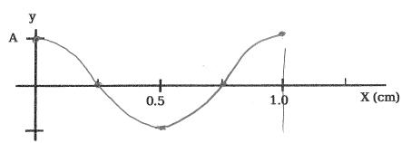
d) (3 pts) Sketch the pressure change, p(x), in the pipe at the same time and conditions as in part (c). P = -B 27
