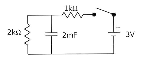
9. The 2mF capacitor has no charge on it before the switch is closed. What is the current through the  $1k\Omega$  resistor at the instant the switch is closed?
