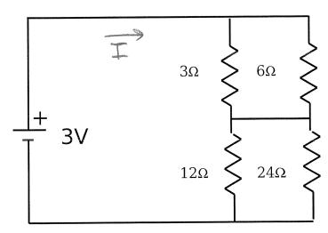
Find the current that is going through the  $3\Omega$  resistor.
