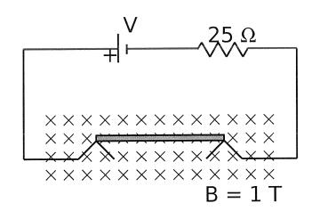
A thin, 50 cm long conducting bar with mass 750g rests on two conducting supports in a uniform 1Tesla magnetic field, as shown above. A battery and a  $25\Omega$  resistor are in series with the supports. The conducting bar completes the circuit, so long as it touches the two conducting supports.
