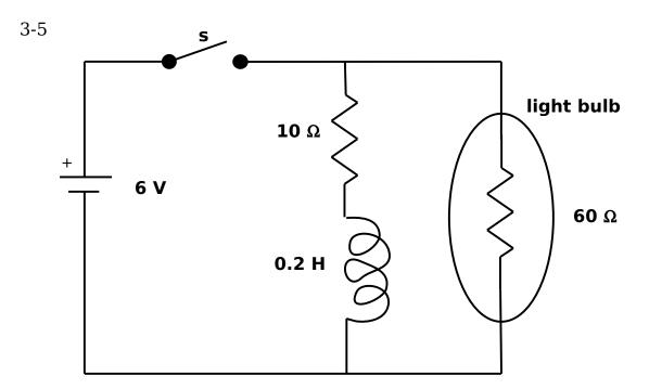
As in a lecture demonstration: After a long time the switch,  ${\bf s},$  above, is closed.
