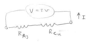
$$V = IR_{Ag} + IR_{cu} \Rightarrow I = \frac{V}{R_{Ag} + R_{cu}} = \frac{V}{\frac{P_{Ag} L_{Ag}}{\pi d^2} + \frac{P_{cu}L_{cu}}{\frac{\pi}{4}d^2}}$$
