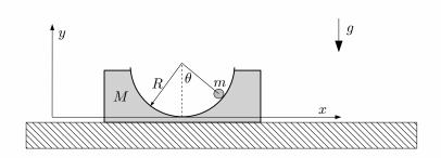
The figure above shows a particle with mass m that slides on a frictionless circular slide. The circular slide has a radius R. The circular slide is cut from a block of that slides without friction on a flat table. The mass of the circular slide block is M. There is a uniform gravitational field with magnitude q.
