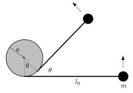
A tether-ball post has a radius a. A small ball with mass m swings on the end of the massless stretch-less rope. The length of the rope decreases as the angle  $\theta$  increases, as the ball gets closer to the pole. Consider all the motion to be in the horizontal plane, so the effect of gravity is ignored. Think of it as a tether-ball on a smooth floor. The length of the rope when  $\theta$  is zero is  $l_0$ .
