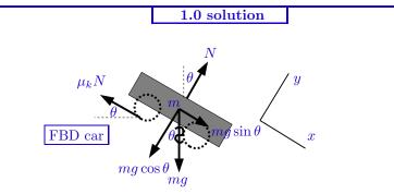
The above figure shows a free body diagram (FBD) of the car. We let m be the mass of the car. Applying Newton's 2nd law gives
