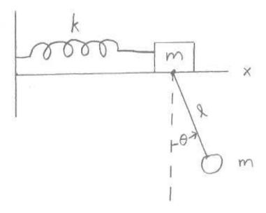
This figure shows a block that slides without friction on a plane with a simple pendulum attached to the bottom of it. All motion is in the plane of this paper. It is given that  $\frac{k}{m} = \frac{g}{l} = \omega_0^2$ , where g is the acceleration due to gravity. Find the normal modes of oscillation and their angular frequencies in terms of the coordinates  $(q_1 \quad q_2) = (x \quad l\theta)$ .
